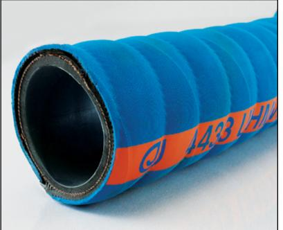
**CONSTRUCTION:** Tube is an Ultra-High Molecular Weight Polyethylene (UHMWPE). Cover is EPDM, blue and corrugated. Reinforcement is a two-ply synthetic fabric with a wire helix.
