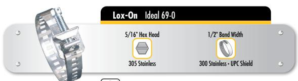
Maximum installation torque of 20 lbf-in (2.25 Nm) / Minimum destructive torque is band failure
