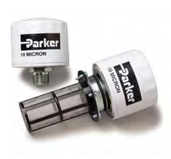
PV Series is an economical Pressure/Vacuum Relief Valve used to maintain positive pressure in hydraulic reservoirs. The large filter area makes this valve an ideal choice for use in heavily contaminated environments. The optional bayonet type mount allows the valve to be installed in the tank filler port, eliminating the need for an extra port. In this configuration, the valve also serves as a filler cap.
