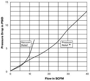
\*Pressure drop is pressure relief valve crack pressure until pressure drop curve increases above pressure relief crack pressure.
