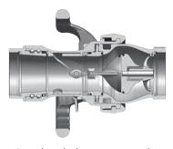
Coupling halves disconnected
