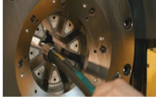
Crimp the hose/fitting assembly.
