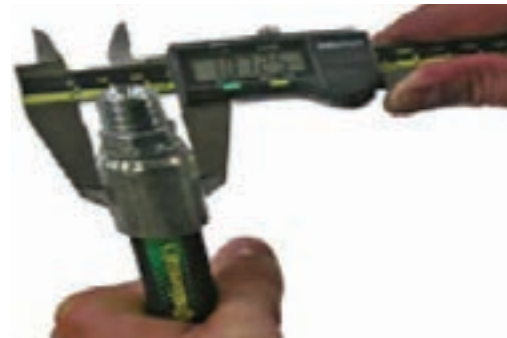
Verify crimp diameter with calipers.
