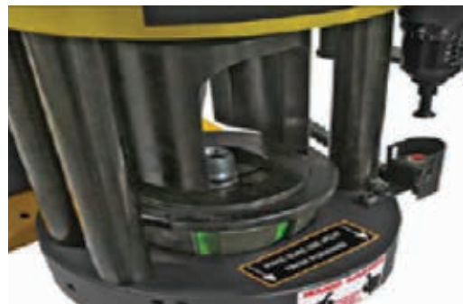
Insert hose assembly into crimper die set.
