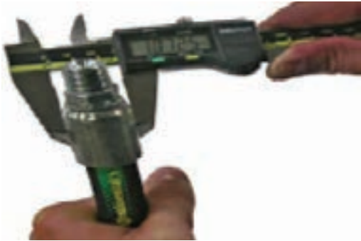
Verify crimp diameter with calipers.
