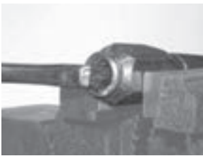
Apply lubricant to stem and hose tube.
