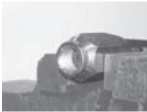
Visually check hose position inside socket.
