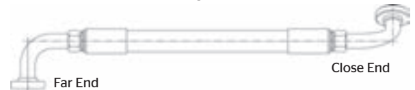
Far End Reference Measuring Clockwise
