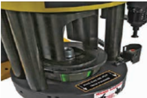
Insert hose assembly into crimper die set.
