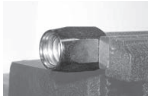
Socket positioned in vice.
