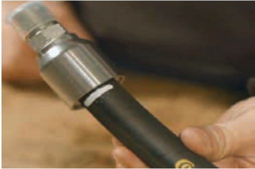
Fitting inserted on hose.
